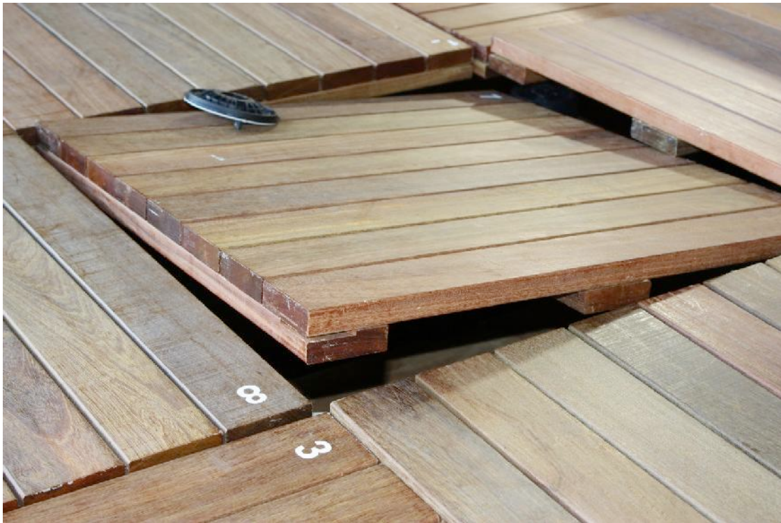
Figure 10 - Tilted paver after wind test. A loose pedestal plate cap may be seen on top of the paver. Shaking of the pavers loosens the caps and when the pavers start lifting allow the wind to pick up the plates. After that pavers no longer have the adequate support
