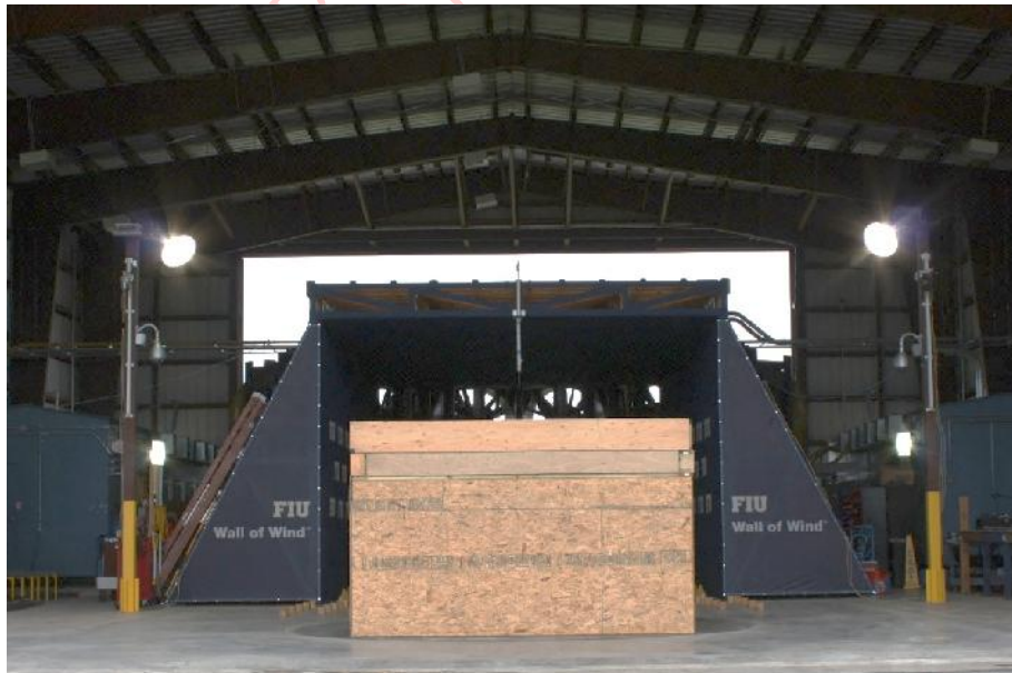
Figure 2 - Base building with 9 in. parapet + 12 in. parapet on top of test section (looking upwind)
