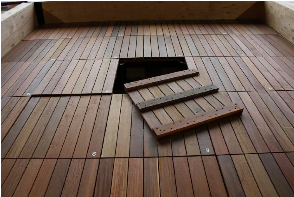
Figure 4 - Blown off wood paver at the parallel slats, 0 degree, 12-in parapet configuration
