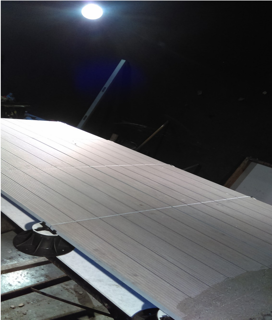
Photograph 1: Perpendicular, Porcelain pavers Prior to Testing
