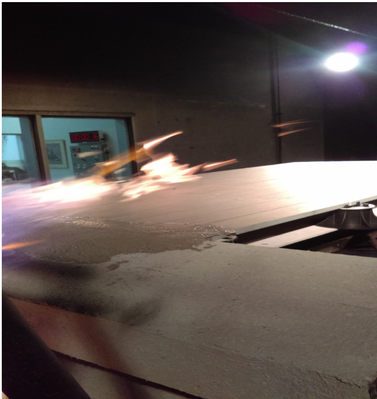
Photograph 2 Perpendicular, Porcelain pavers at Maximum Flame Spread
