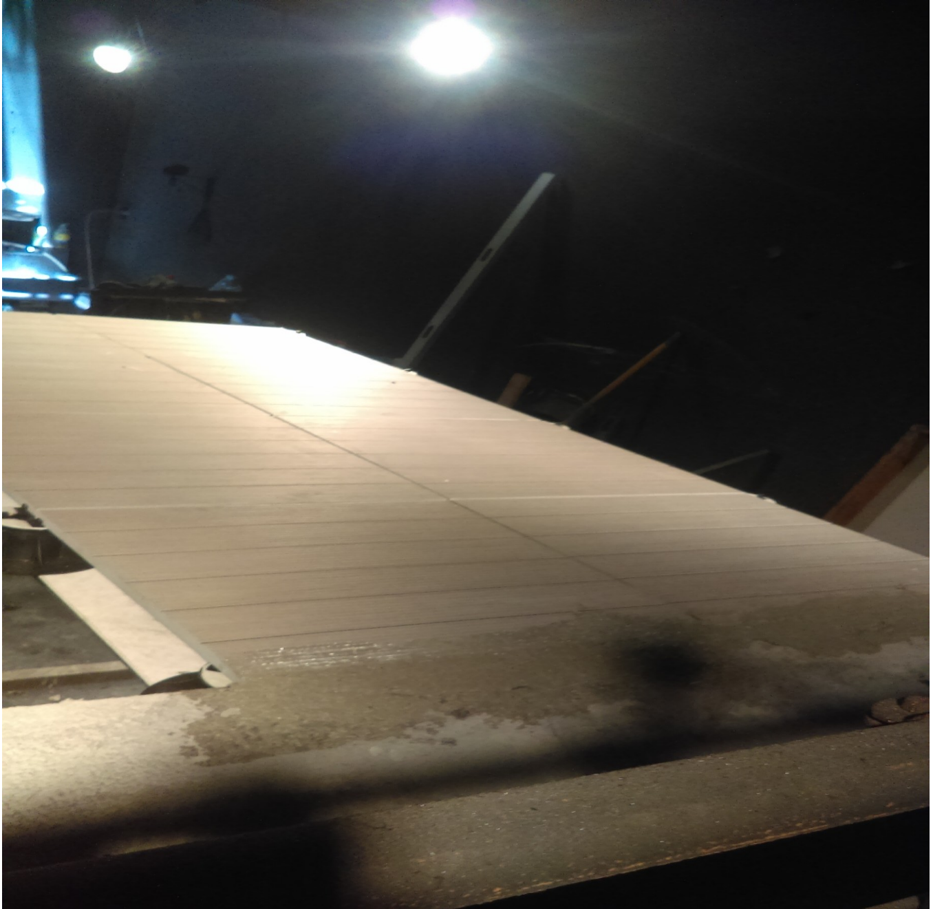
Photograph 4: Parallel Porcelain pavers Prior to Testing
