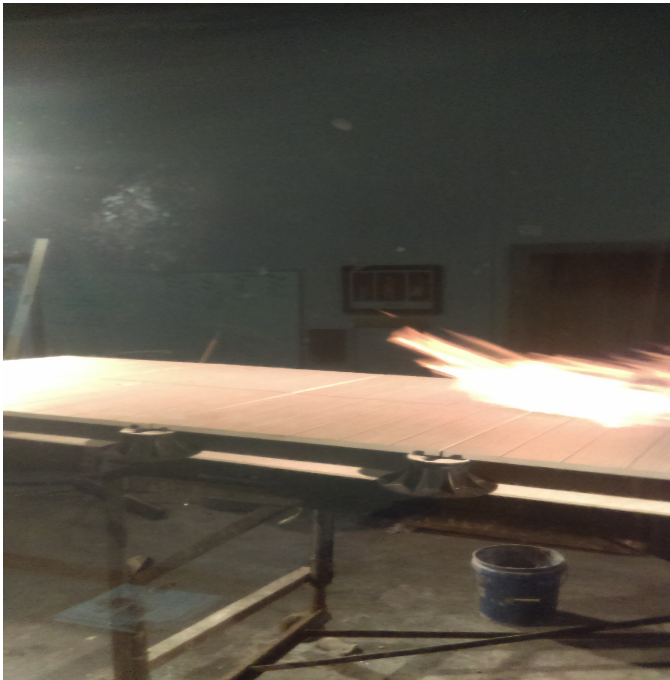
Photograph 5 Parallel, Porcelain pavers at Maximum Flame Spread
