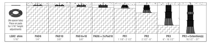
For heights over 16 1/2", screw extension element (7") onto PR 3 pedestal between lower and upper columns. Do not exceed heights of 23" with 1 x extension, 30" with 2 x extensions and 37" with 3 x extensions. Guy wires or other approved bracing should be used for pedestal heights above 24". On heights over 16 1/2" consult with our sales team if extra stablization is needed.
