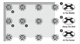
Break off unneeded spacer tabs. At corners of deck area, make an additional cut on base of pedestal at right angles to existing cut.
