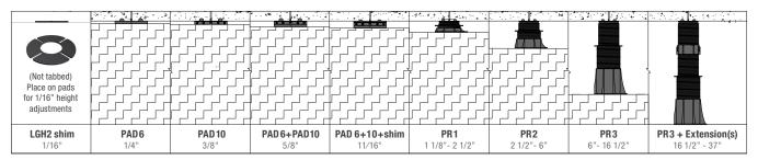
For heights over 16 1/2", screw **extension elements** onto PR 3 pedestal between lower and upper columns. Do not exceed heights of 23" with 1 x extension, 30" with 2 x extensions and 37" with 3 x extensions. Guy wires or other approved bracing should be used for pedestal heights above 24". On heights over 16 1/2" consult with our sales team if extra stablization is needed.
