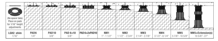
For heights over 10 5/8", screw extension element (6 1/2") onto NM5 pedestal between lower and upper columns. Do not exceed heights of 16" with 1 x extension, 21" with 2 x extensions and 27" with 3 x extensions. Guy wires or other approved bracing should be used for pedestal heights above 24". On heights over 10 5/8" consult with our sales team if extra stablization is needed.
