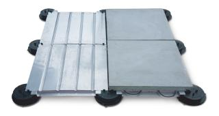
Aluminum support brackets, 4" wide, are laid between adjustable height pedestals to support polyurethane foam insulation. Aluminum trays, with pre-adhered insulation and V-shaped channels for the heating element, are placed on the brackets.
