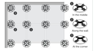
Break off unneeded spacer tabs. At perimeter walls, cut one side of base along the scored lines. At corners, make an extra cut on base at right angles to first cut.
