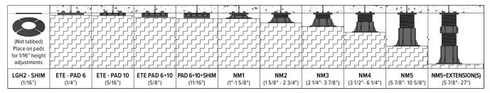
For heights over 10 5/8", screw **extension elements** onto NM5 pedestal between base and screwed column. Do not exceed height of 16" with 1 x extension, 21" with 2 x extensions and 27" with 3 x extensions. Guy wires or other approved bracing should be used for pedestal heights above 24".
